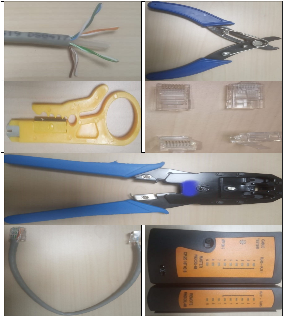
Figure 2.13: RJ-45 Connector, Twisted Pair Cable, and Tools
